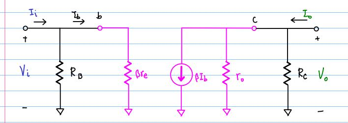
$$Z_i = R_B || \beta r_B \cong \beta r_B \qquad (R_B) || \log r_B)$$
