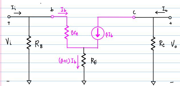
$$\begin{aligned} &\mathcal{E}_{i} = R_{B} \| \mathcal{F}_{b} \cong R_{B} \| \beta (re + R_{E}) \cong R_{B} \| \beta R_{E} \\ &\mathcal{E}_{0} = R_{C} \\ &V_{0} = -\beta I_{b} R_{c} = -\beta \left(\frac{V_{i}}{Z_{b}}\right) R_{C} \\ &A_{v} = \frac{V_{0}}{V_{i}} = -\frac{\beta R_{c}}{Z_{b}} = -\frac{\beta R_{C}}{\beta (re + R_{E})} = -\frac{R_{c}}{re + R_{E}} \cong -\frac{R_{c}}{R_{c}} \end{aligned}$$
