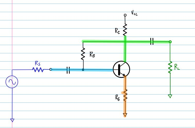
$$A_{V} = -\frac{(R_{L} || R_{c})}{R_{E}} - \frac{(R_{L} || R_{c} || r_{o})}{R_{E}}$$
