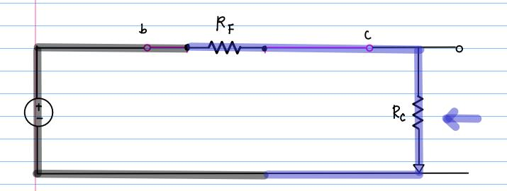
$$Z_{0} = R_{c} \parallel R_{F}$$
