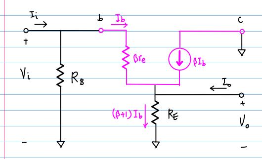
$$I_b = \frac{V_i}{Z_b} \qquad (6+1) I_b = (6+1) \frac{V_i}{Z_b}$$
