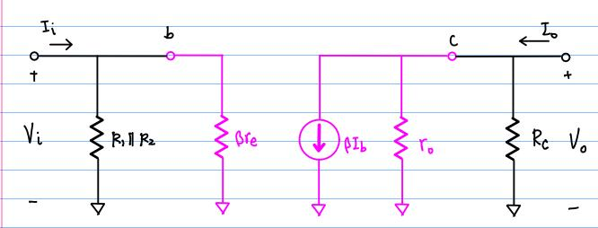
$$Z_i = |R_1||R_2||\beta \Gamma e$$
