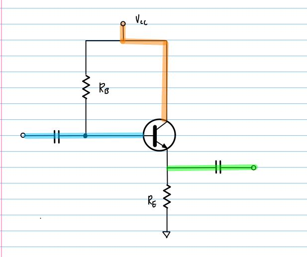
$$Z_i = R_B \parallel \beta(r\acute{e} + R_E) \cong R_B \parallel \beta R_E \qquad \text{High (100 } kS)$$
