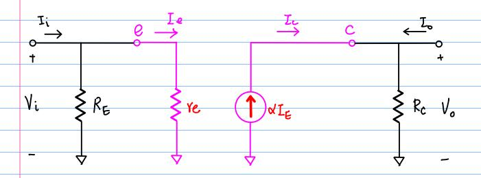
$$A_{V} = \frac{V_{o}}{V_{i}} = \frac{\propto R_{c}}{r_{e}} \cong \frac{R_{c}}{r_{e}}$$
