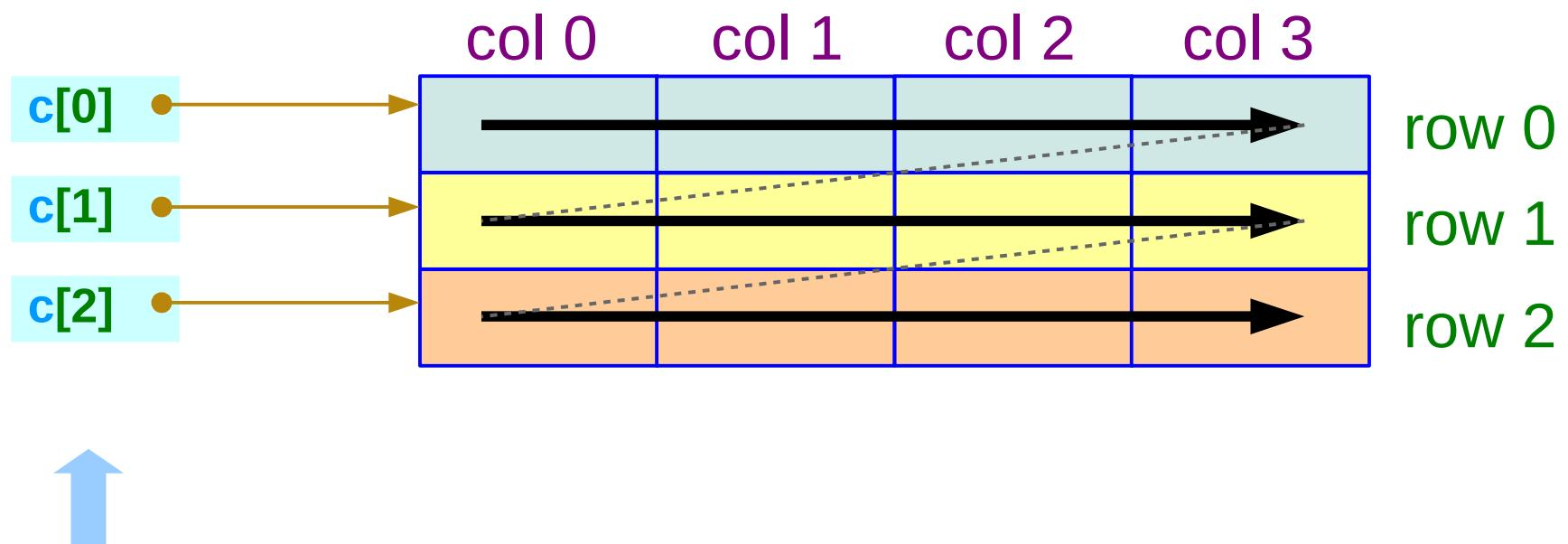
consider each `c[i]` as a pointer to the first element of each 4 element array
