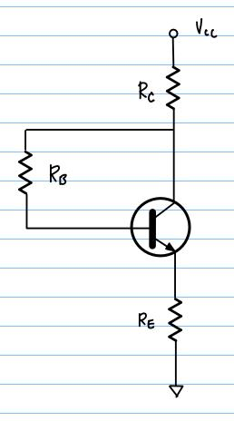
$$T_{B} = \frac{V_{cc} - V_{BE}}{R_{B} + \beta(R_{C} + R_{E})}$$
