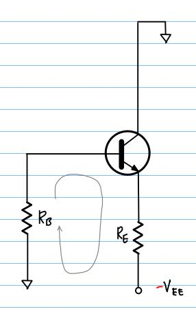
$$I_{B} = \frac{V_{EE} - V_{BE}}{R_{B} + (6+1) R_{E}}$$
