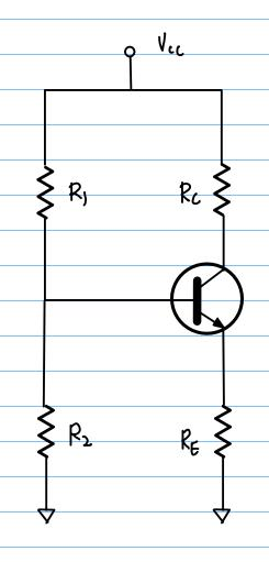
$$V_{0} = \frac{R_{2}}{R_{1} + R_{2}} V_{cc}$$
