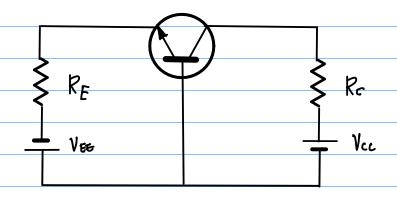
$$I_{E} = \frac{V_{EE} - V_{BE}}{R_{E}}$$
