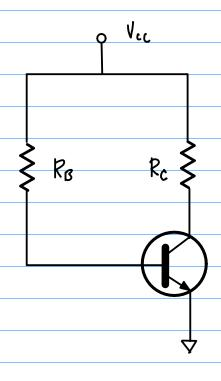
$$I_{B} = \frac{V_{CC} - V_{BE}}{k_{B}}$$
