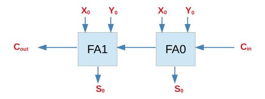
Unless the two FA's are in propagate mode, the transition of Cin does <u>not</u> affect the transition of Cout
