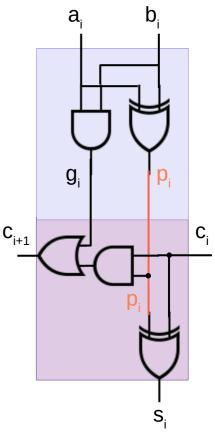
The critical path of a Carry Skip Adder begins at the first full adder, passes through all adders and ends at the sum bit  $s_{n-1}$
