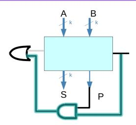
If all n/4 blocks propagate, a carry entering the least significant stage will pass to the most significant carry-out in time n/4 times the delay through the carry-skip unit
