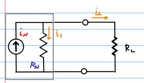
$$i_{l} = \frac{R_{L}}{R_{N} + R_{L}} i_{N}$$
