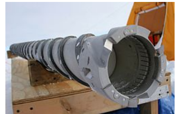
Figure 2 | Mechanical ice auger, showing cutting teeth, helical flights used to transport ice cuttings up away from the cutting region, and a central void for the core itself Steven Profaizer, National Science Foundation, public domain
