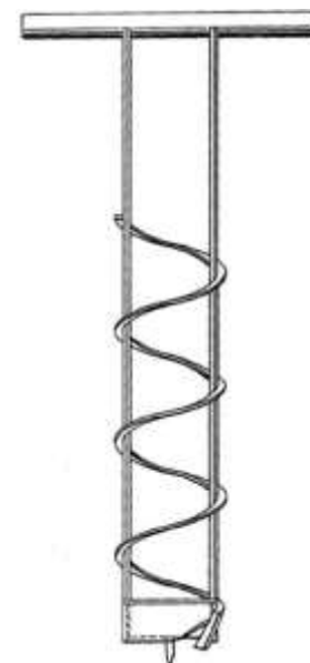
Figure 5 | Coring ice auger with no barrel. Designs like this proved difficult to make sufficiently rigid. [31] Talalay (2016)
