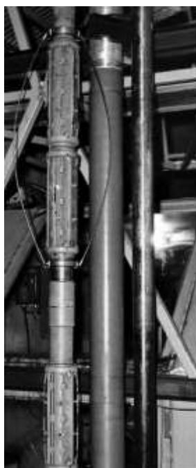
Figure 13 | Leaf springs and hinged friction blades on CRREL drill used to drill at Byrd Station in Antarctica from 1966 to 1968. Talalay (2014)
