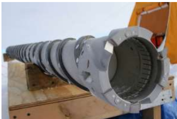
Figure 2 | Mechanical ice auger, showing cutting teeth, helical flights used to transport ice cuttings up away from the cutting region, and a central void for the core itself.
