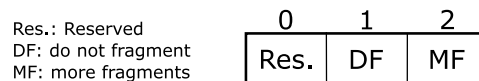
Figure 7: The structure of Flags field in the IPv4 header. CC BY SA 4.0
