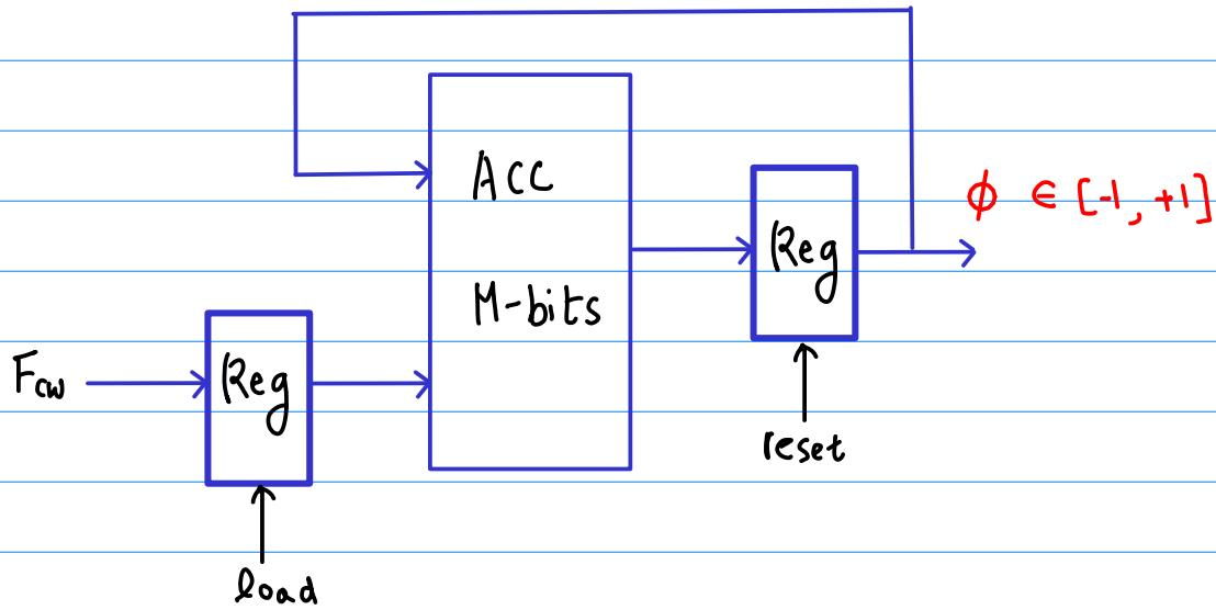
**M-bit** adder - repeatedly increments the phase a
