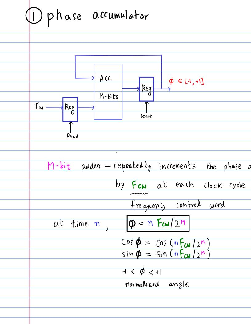
Normalized Angle at time n,  $\varphi = \eta F_{cw}/2^{M}$  $\cos \phi = \cos \left( \frac{nF_{cw}}{2^{m}} \right)$   $\sin \phi = \sin \left( \frac{nF_{cw}}{2^{m}} \right)$  $\phi$  radians/TI  $-| < \phi < +|$  $\pi \phi$  radians -∏< Q < +∏ **b** radians  $\phi = \pi \phi$ Ø∈ [-∏, +∏] Ø e [-1,+1]
