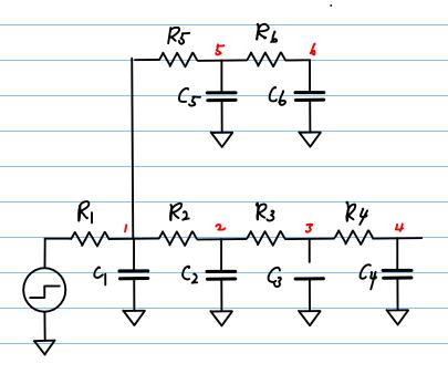
$t_{pd3} = R_1C_1 + (R_1 + R_2)(2 + (R_1 + R_3 + R_3)(3 + (R_1 + R_2 + R_3)(4 + R_1 C_5 + R_1 C_6)$   $t_{pd5} = R_1C_1 + R_1C_2 + R_1C_3 + R_1C_4 + (R_1 + R_5)(5 + (R_1 + R_3)C_6$
