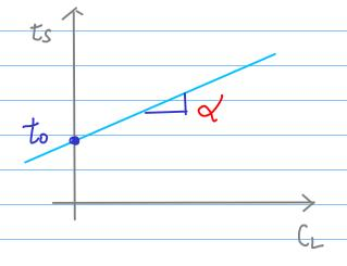
to: zero delay x: slope
