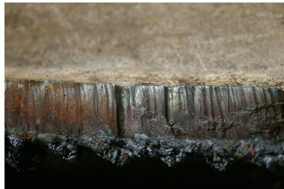
Freehand cut of a thick steel plate
