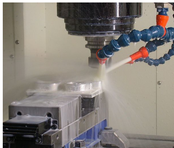
Thin wall milling of aluminum using a water based cutting fluid on the milling cutter
