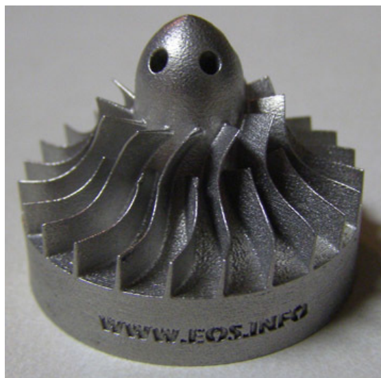
Model of a turbine showing the benefits of 3d printing in industry
