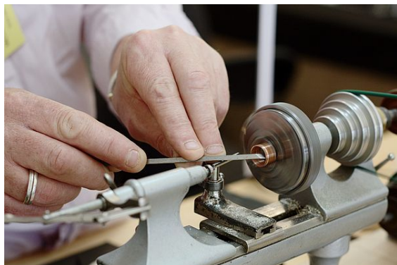
A watchmaker using a lathe to prepare a component cut from copper.
