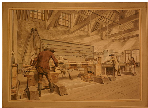
Exact drawing made with camera obscura of horizontal boring machine by Jan Verbruggen in Woolwich Royal Brass Foundry approx 1778 (drawing 47 out of set of 50 drawings)
