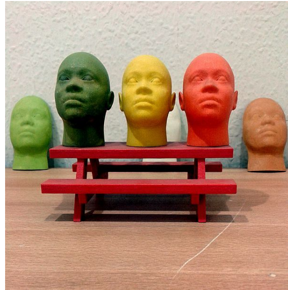
Miniature face models (from FaceGen) produced using several colored plastics on a 3D Printer
