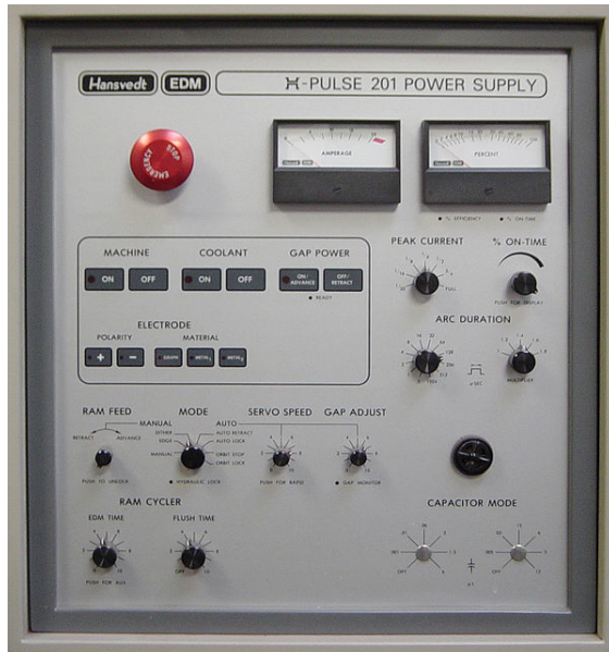
EDM control panel (Hansvedt machine). Machine may be adjusted for a refined surface (electropolish) at end of process.
