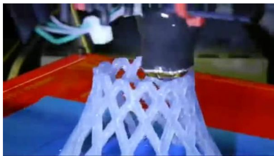
Timelapse video of a hyperboloid object (designed by George W. Hart) made of PLA using a RepRap "Prusa Mendel" 3 printer for molten polymer deposition
