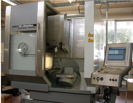
Five-axis machining center with rotating table and computer interface
