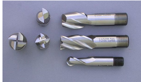
High speed steel with cobalt endmills used for cutting operations in a milling machine.
