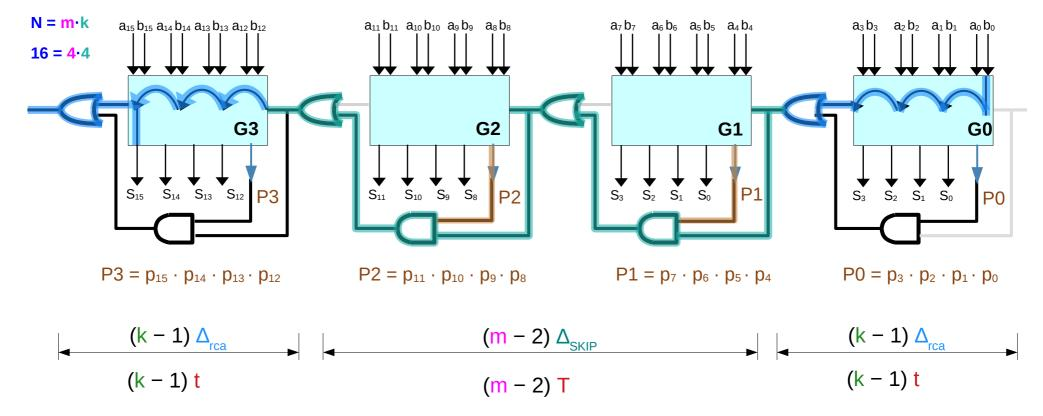
*t* denote the time required for a carry signal to ripple across a bit *T* denote the time required for the signal to skip over a group of bits *m* denotes the optimal number of groups for an n-bit carry chain
