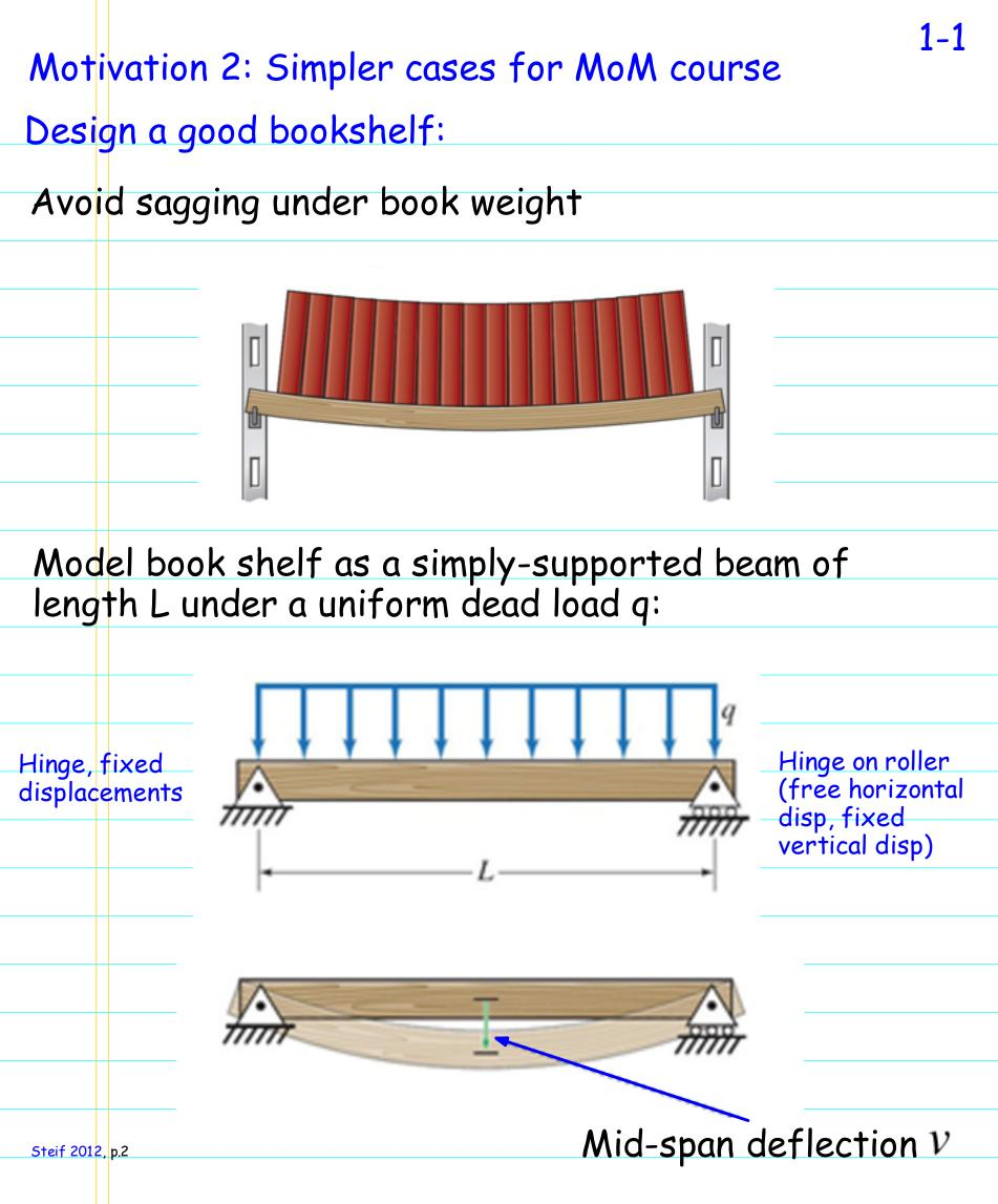
How to estimate the deflection V in terms of the beam length L and the distributed load q, and the properties of the material used for the shelf?
