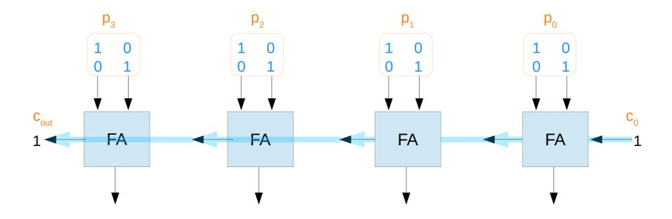
$c_0$  can be propagated to  $c_{out}$  only when s = 1
