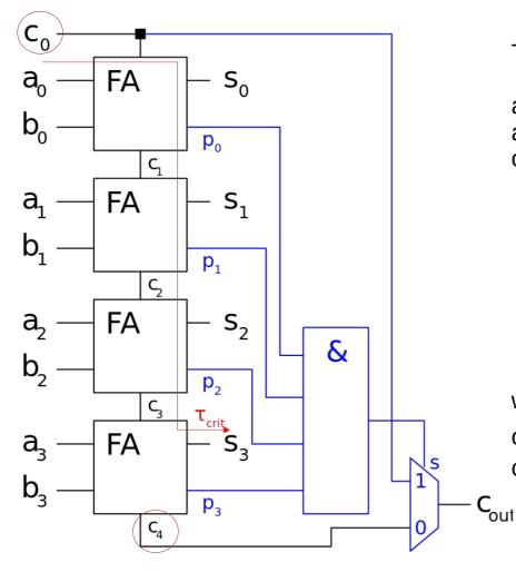
The n-bit-carry-skip adder consists of
