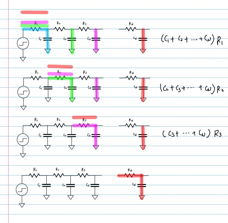
$$t_{pd} = P_{1} \left( C_{1} + (c_{2} + \cdots + c_{N}) + P_{3} \left( c_{2} + c_{3} + \cdots + c_{N} \right) + P_{3} \left( c_{3} + c_{4} + \cdots + c_{N} \right) + \cdots + P_{N} C_{N} \right)$$
