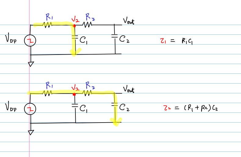
$$7 = 7_1 + 7_2 = [R_1C_1 + (R_1 + R_2)C_2]$$
