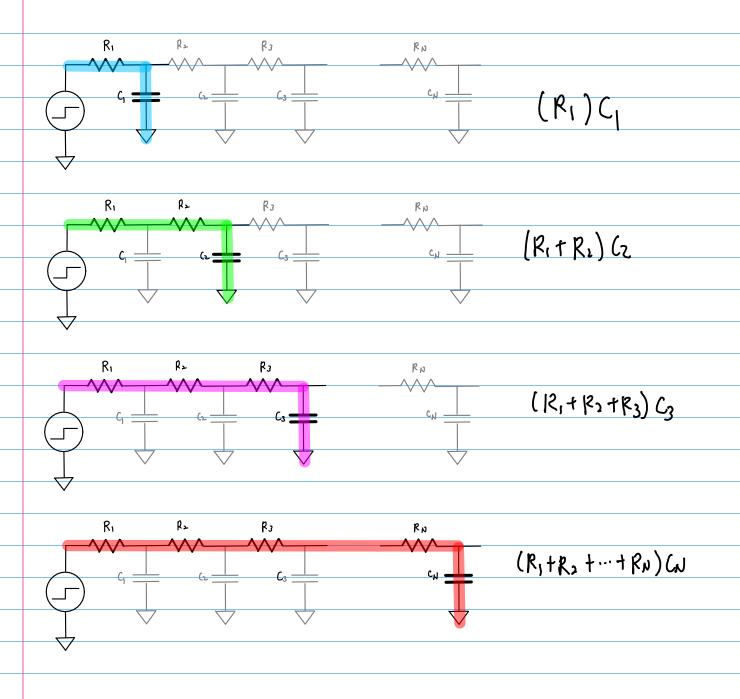
$$t_{pd} = \sum_{i=1}^{n} \left( \sum_{j=1}^{l} R_{j} \right) C_{i}$$
