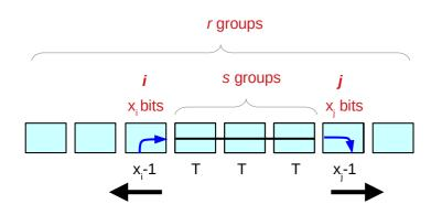
A signal <u>originating</u> in group i, <u>rippling</u> to the end of this group i and then skipping over the next s group has delay  $(x_i - 1) + sT$
