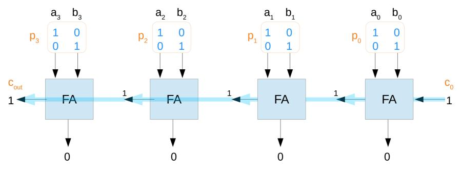
$c_0$  can be propagated to  $c_{out}$  only when s = 1
