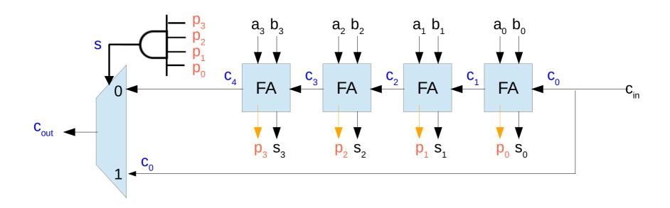
The n-bit Carry Skip Adder consists of
