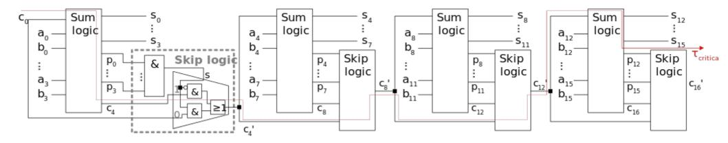
Since the Cin-to-Cout represents the longest path in the ripple-carry-adder, an obvious attempt is to accelerate carry propagation through the adder.
