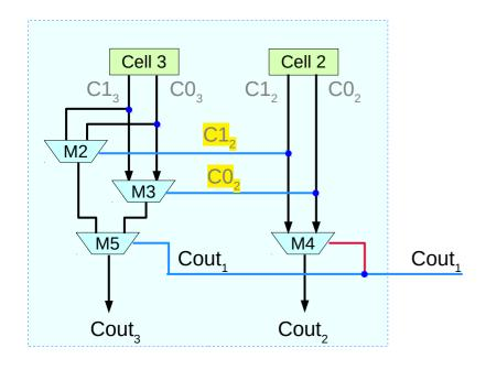
$$(C1_3 C1_2 + C0_3 \overline{C1}_2)Cout_1 + (C1_3 C0_2 + C0_3 \overline{C0}_2)\overline{Cout}_1$$
