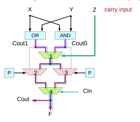
a delay of 3 in the first cell 1 in mux1, 1 in mux2, 1 in mux4
