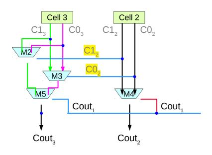
$$(C1_3C1_2 + C0_3\overline{C1}_2)Cout_1 + (C1_3C0_2 + C0_3\overline{C0}_2)\overline{Cout}_1$$
