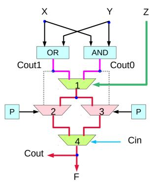
For the <u>first</u> cell in a carry chain with a <u>carry input</u> (provided by input Z), <u>mux2</u> and <u>mux3</u> both pass the value from <u>mux1</u>
