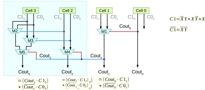
$$C1 = \overline{X}Y + X\overline{Y} + XY$$
