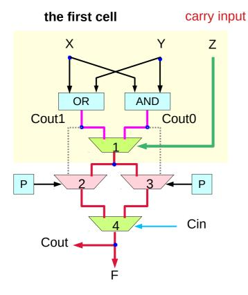
mux1's main inputs are driven by two 2-LUTs (OR, AND) controlled by X and Y mux1 forms a **3-LUT** with the other 2-LUTs
