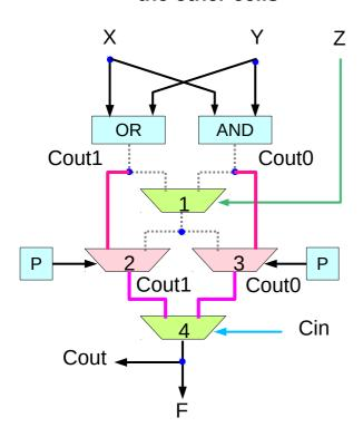
for cells in the middle of a carry chain mux2 passes Cout1 mux3 passes Cout0 mux4 receives Cout1 and Cout0 provides a standard ripple carry path.
