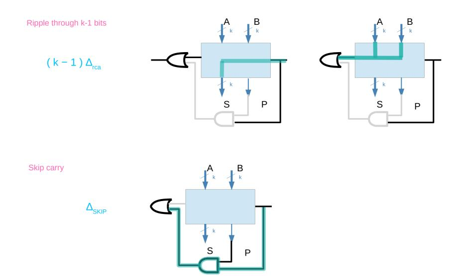
The <u>maximal delay</u>  $\Delta$  of a Carry Skip Adder is encountered <u>when carry</u> is generated in the <u>least-significant bit</u> position,
